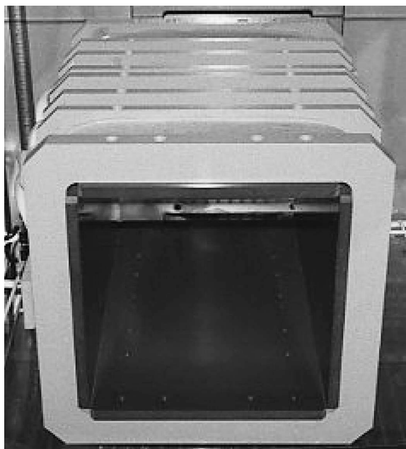
Fig. 1. The EMF generator systems. The experimental magnetic fields coils to generate horizontal sinusoidal EMFs of 50-Hz, 10-mT (218×218×387 mm).
