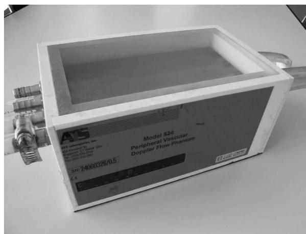
Fig. 1. The tissue-equivalent phantom used in these experiments.
