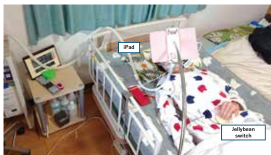
Fig. 2 Using iPad® in bed The iPad® is held in place by a monitor arm and operated with a switch.
