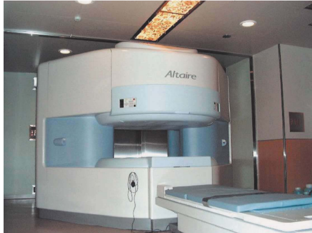
Fig. 1. The picture demonstrates an open type magnetic resonance imaging (MRI) Altaire 0.7T (Hitachi Medical Corporation) installed in Jikei Kashiwa Hospital.
